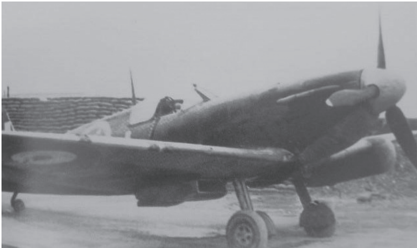
A Spitfire MkIIa with a 40 gallon single port wing fixed fuel tank. [ http://s412.photobucket.com/user/ruspren/media/ruspren001/IMG_0703_zpsa8bob786.jpg.html ]
